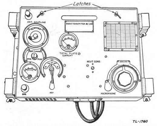
FIGURE 3.—Front panel view of radio transmitter BC-228, a part of radio set SCR-203.
